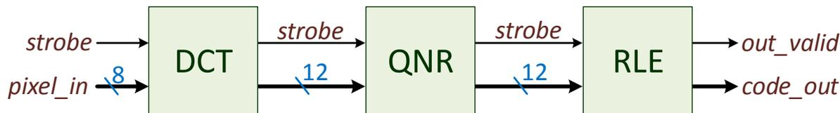
Figure 11.3: Single-stream JPEG block diagram.
